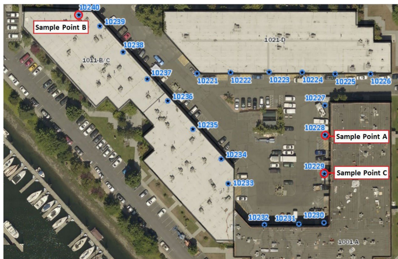
Figure 3. Oyster barrel locations at Terminal 102 displaying the three sample locations (numbered stars are downspouts)
