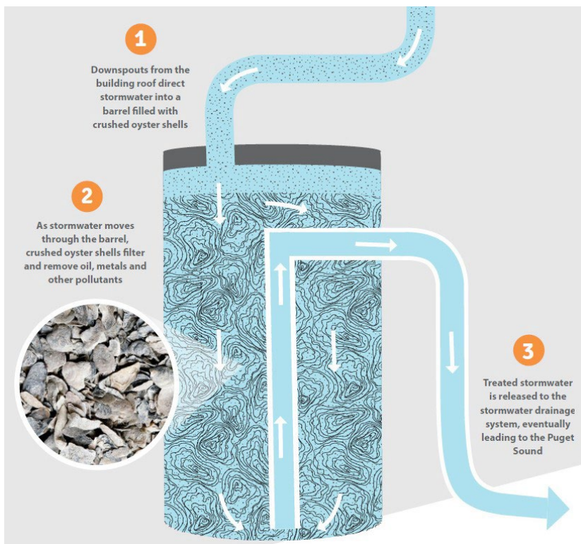
Figure 2. Information sign for oyster shell downspout barrels at Terminal 102
